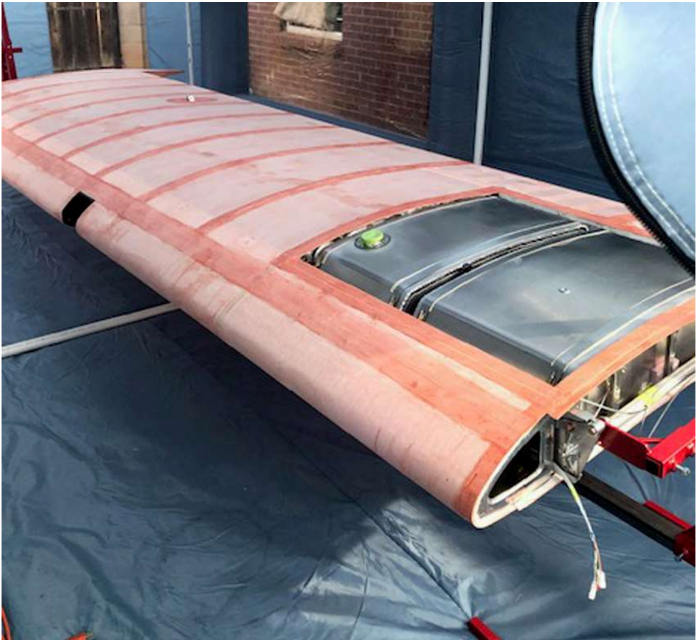
Carbon Cub wing with Fabric Covering
