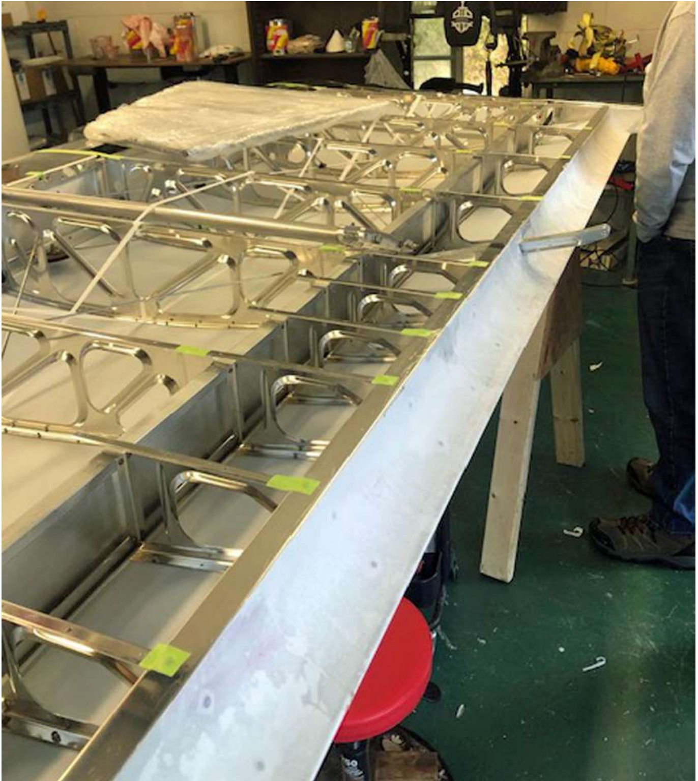
Carbon Cub Wing before Covering
