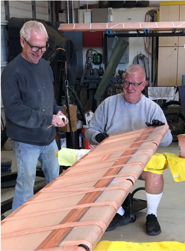
Jack Pollack and Terry Emig having fun rib stitching a Stearman aileron
