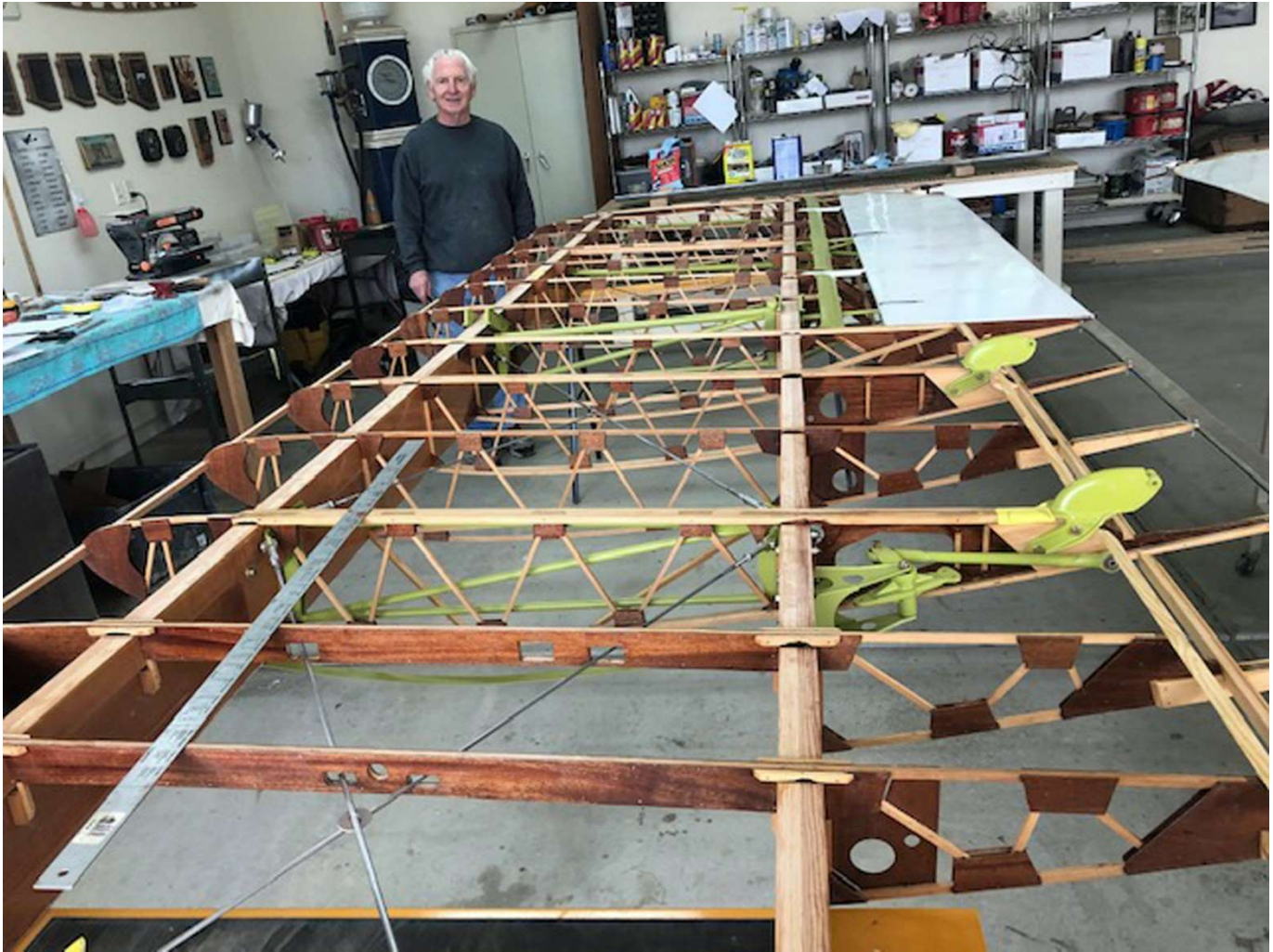
Jack Pollack is making great progress on building a new set of wings for a Fairchild 24. There are a lot of parts in them.
