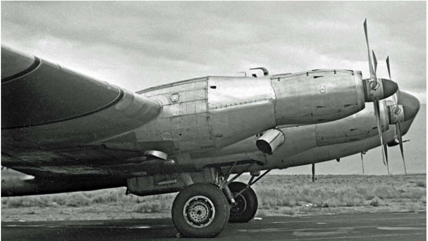
In an effort to make the worlds loudest airplane Rolls Royce Dart engines have been installed on a Boeing B-17
