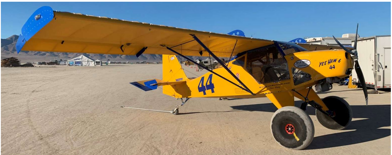
Steve Henry's highly modified Gold Class Racer with a Yamaha 300 hp engine
