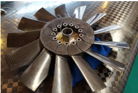
Ducted Axial Fan from the ALBI UL-39
