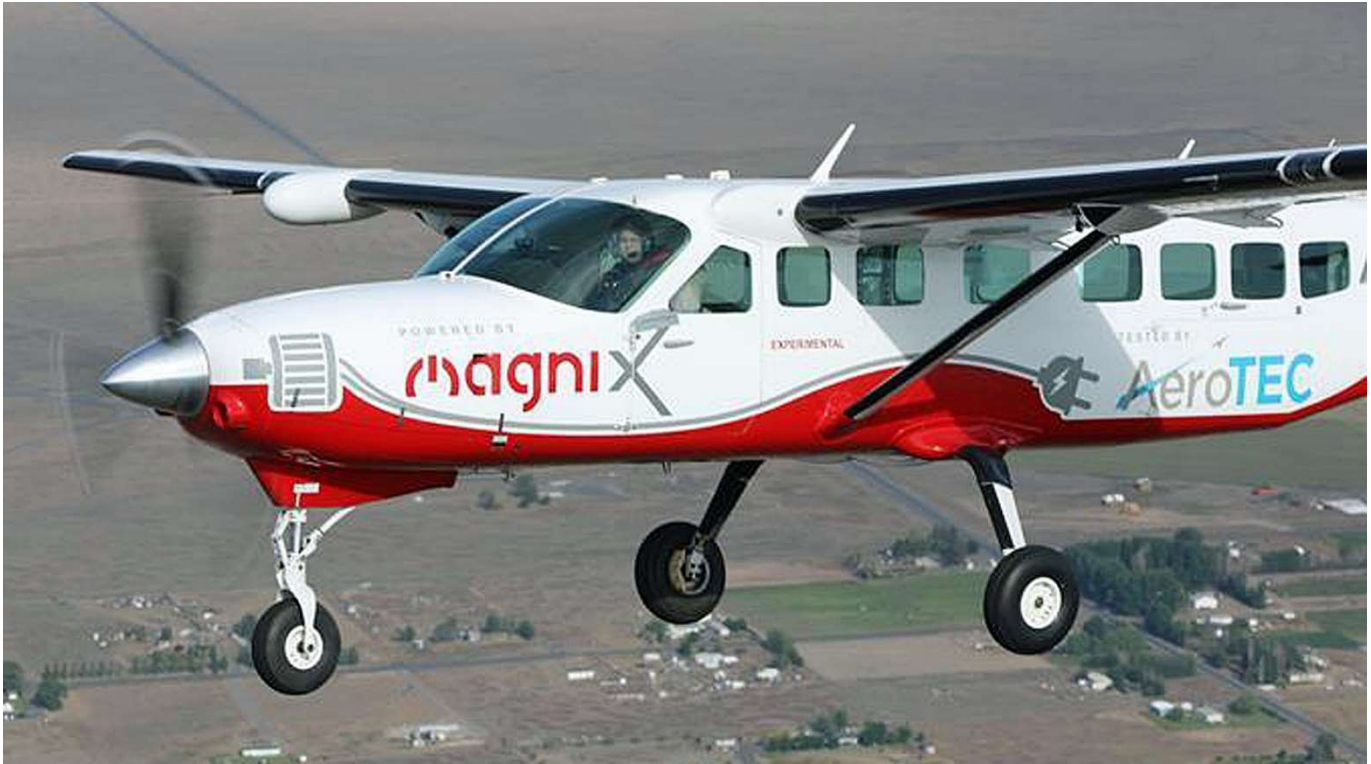
Cessna Grand Caravan with Magnix Electric Power
