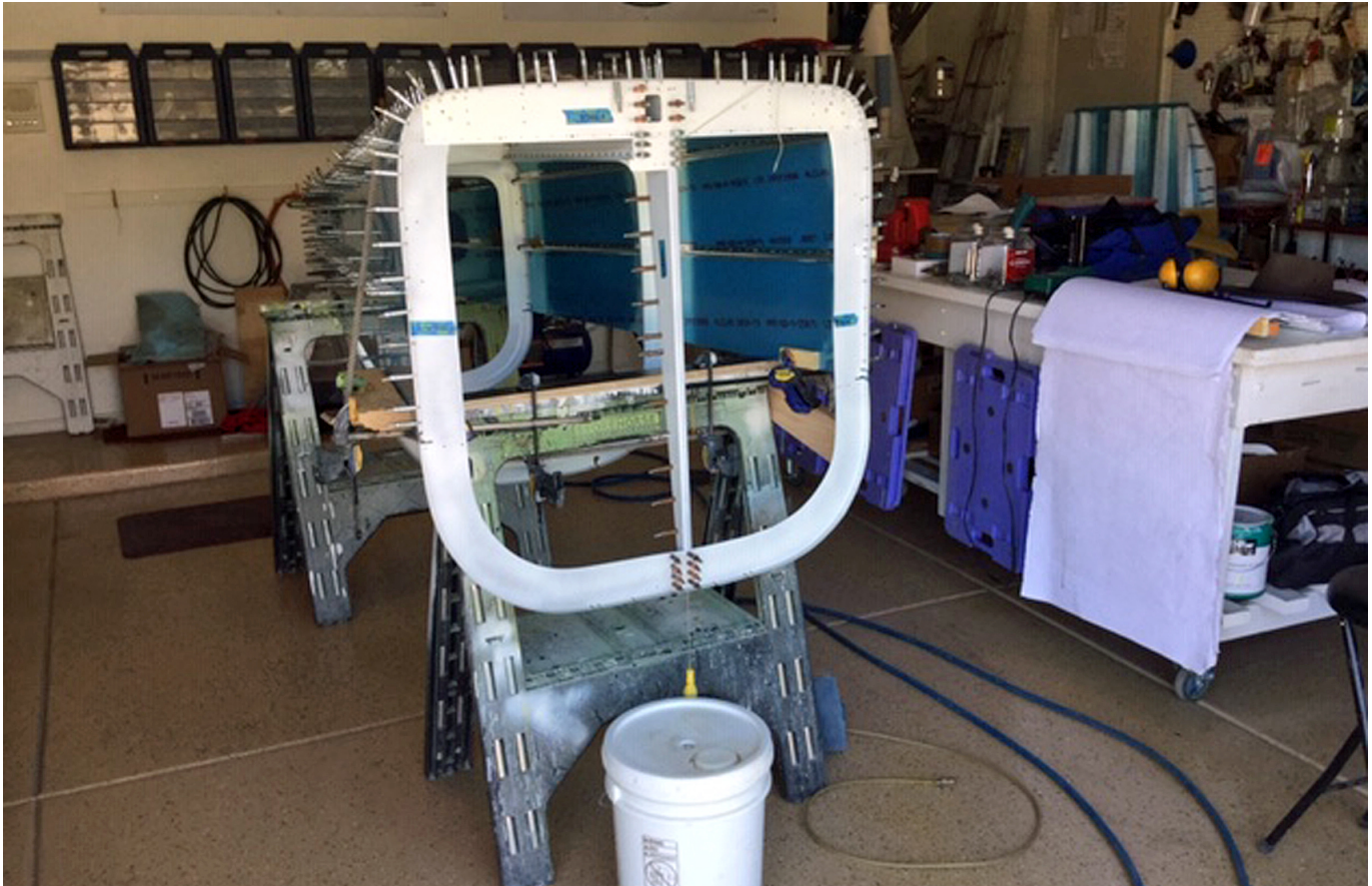
John Davis is building his fourth RV. Here is a picture of the rear fuselage going together. The wings and tail are done and in his hangar at DVT
