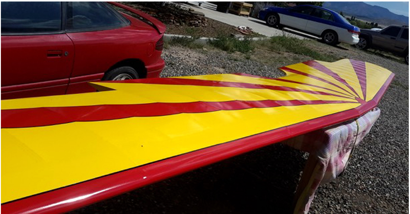
Bill's Upper Skybolt Wing He is Using the Stewart Systems Process for Recovering Them
