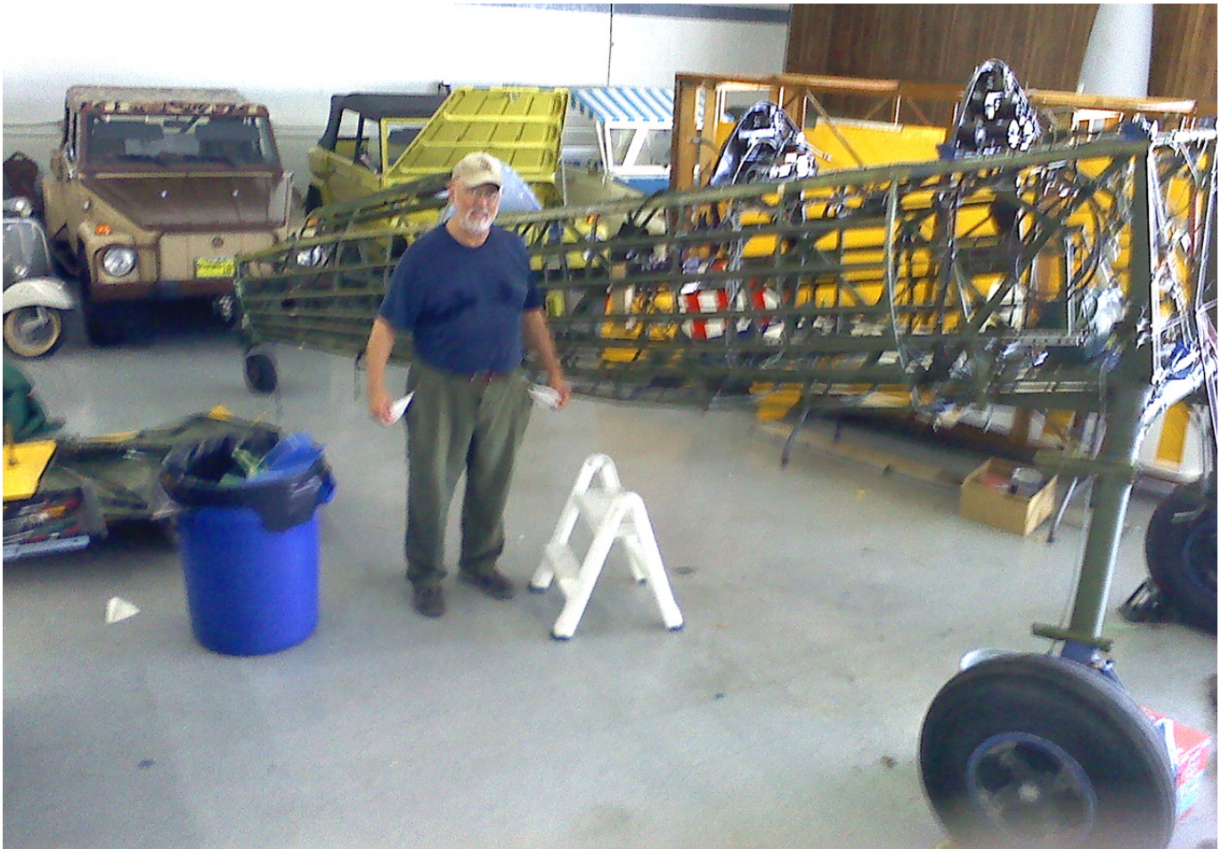
Billy Walker's Stearman N47964 under restoration for New engine and fabric
