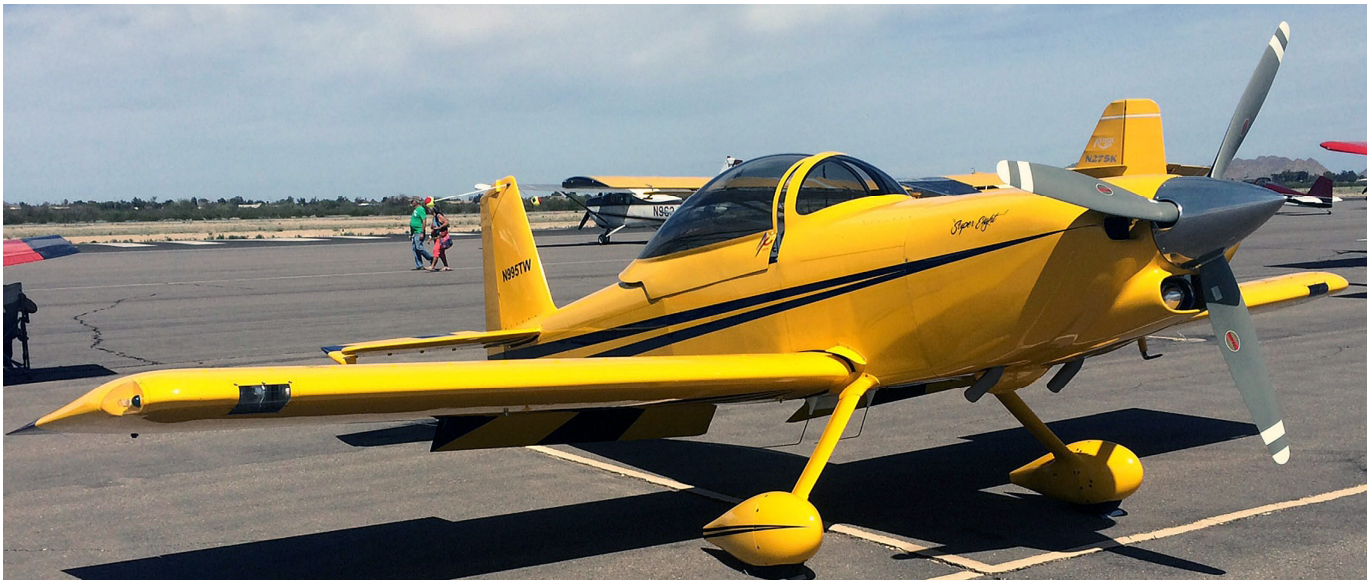
This rare bird is a super RV-8 powered by a 300 hp Lycoming 540. It is owned by Chapter member Bill Lewallen
