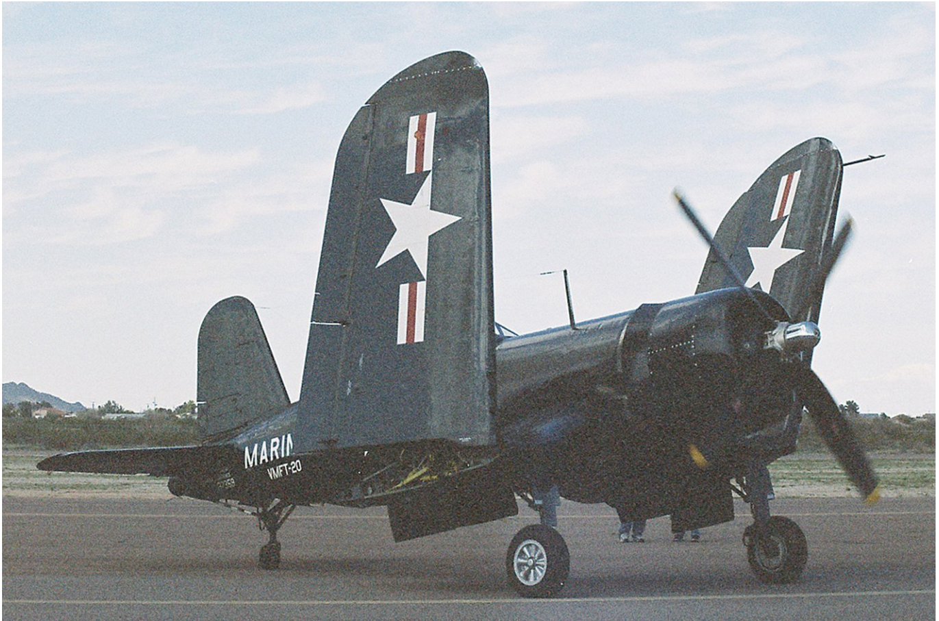
Corsair Demonstrating its Folding Wing Capability while Preparing to Take Off
