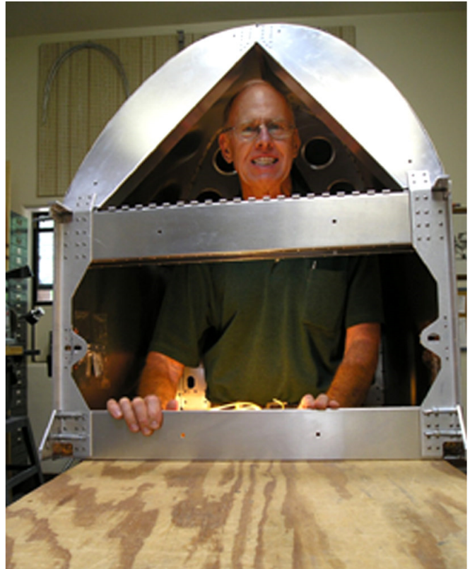
A View of the Aft Fuselage Construction
