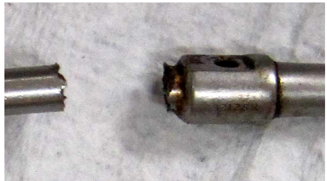
Close Up of Turnbuckle Failure
