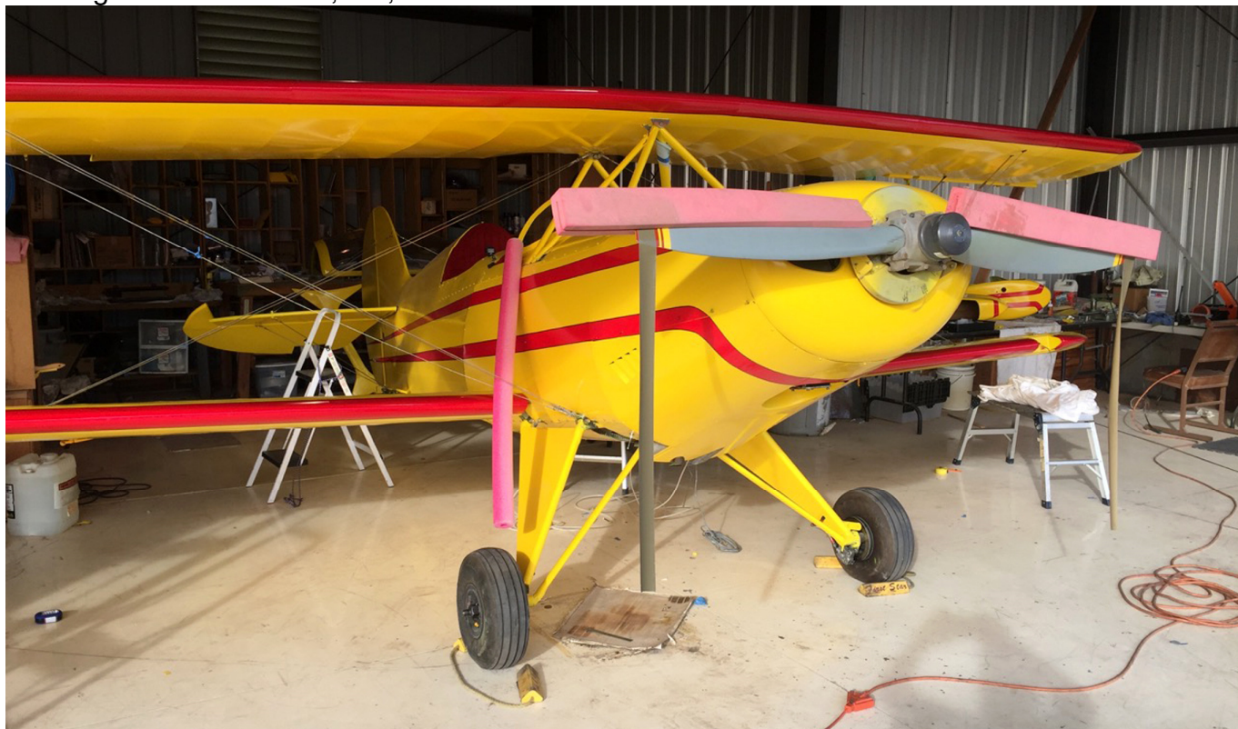
Bill Unternaehrer's Skybolt going back together after Being recovered with Stewart Systems
