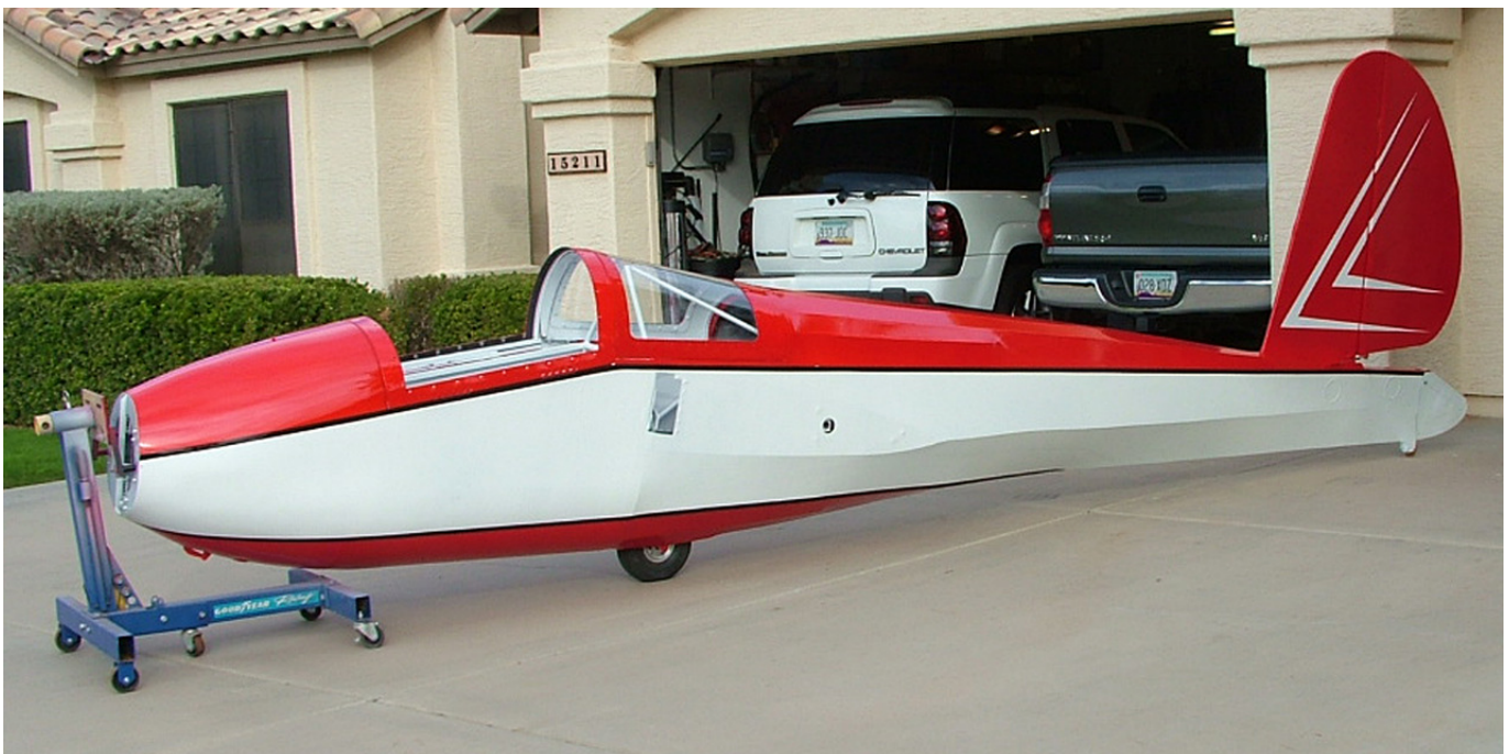
Jerry Lane's Schweizer 1-26 new paint job using Stewart Systems water based process. With no smell he said he could shoot it in his living room, luckily he didn't
