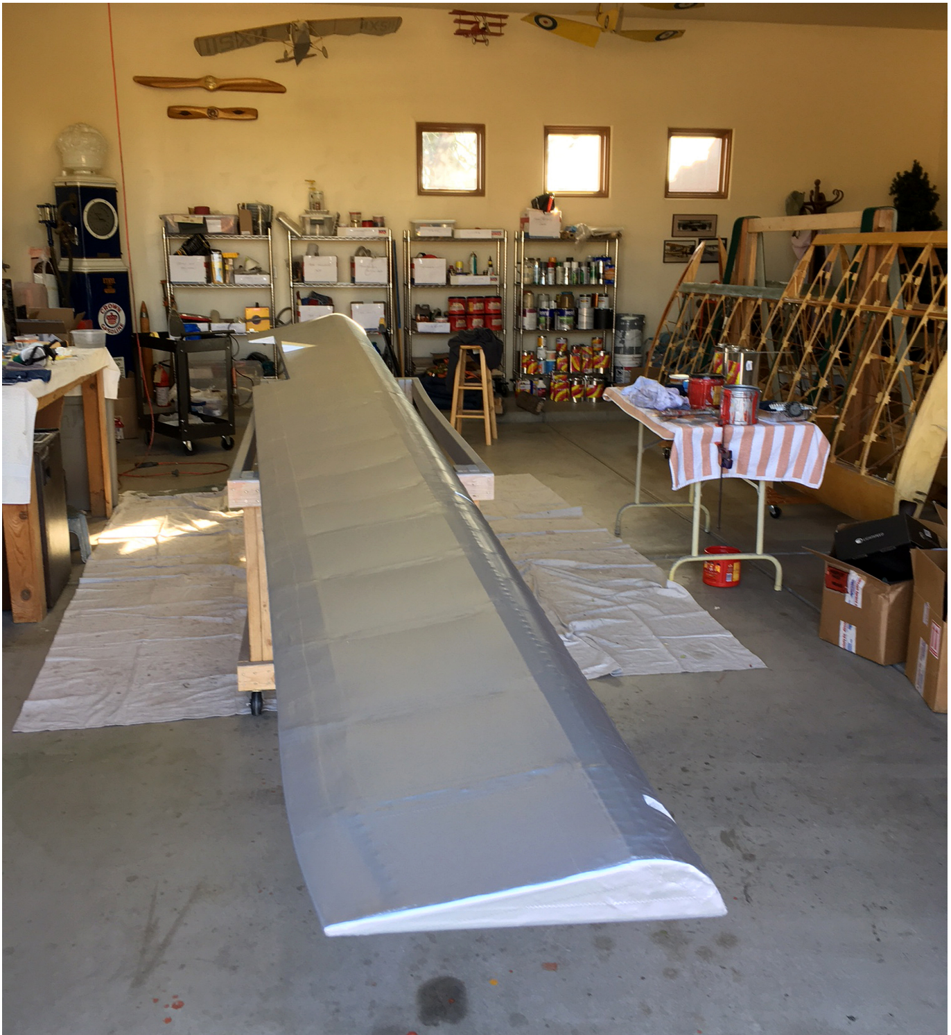
Jack Pollack just finished recovering the Ailerons on a Consolidated PB4-Y2. Each one is 21 feet long!
