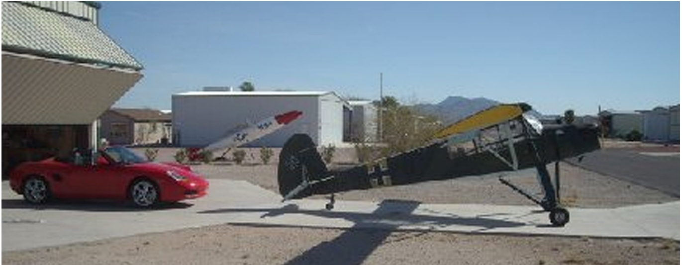
Bernie Gross's Jabiru 2200 powered Fieseler Fi 156 Storch seen at the Carefree 50 year Anniversary Fly-In
