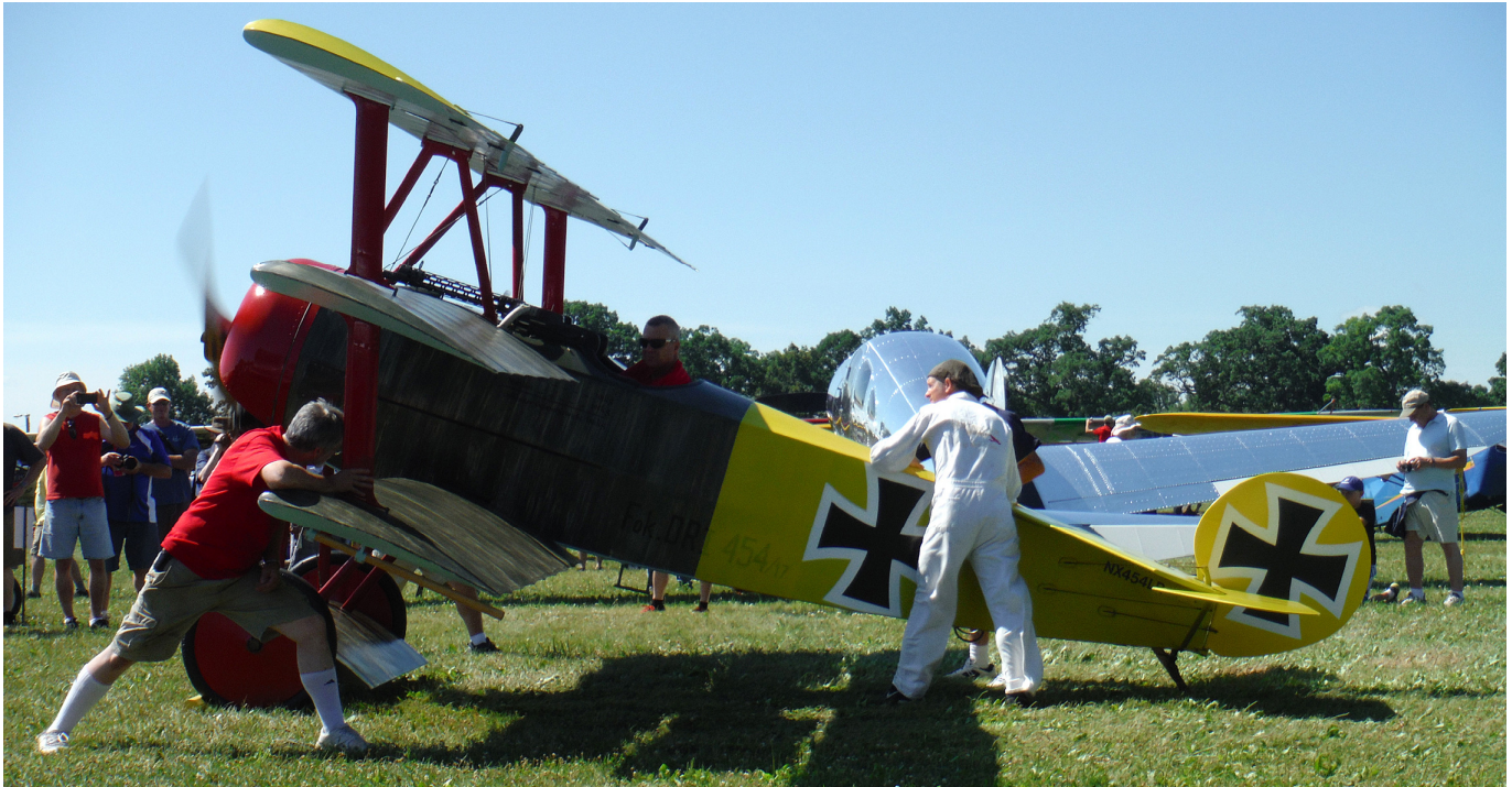
Fokker Triplane Running Up. Engine is Either On or Off, No Throttle
