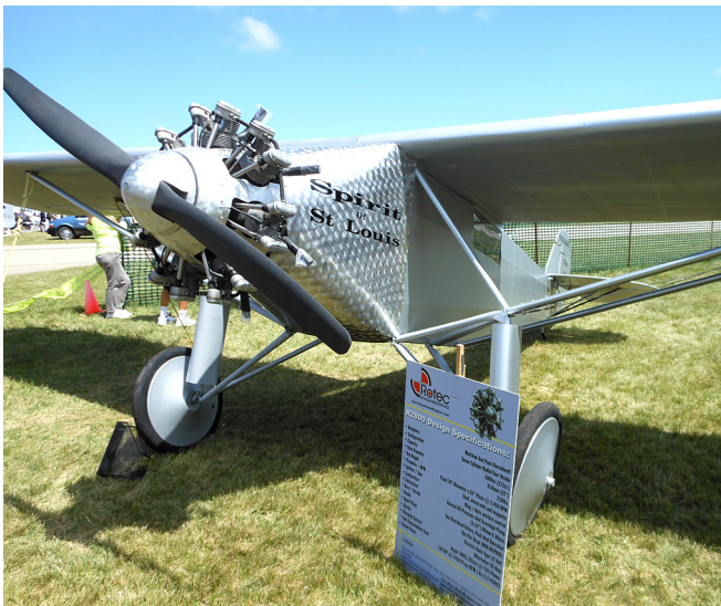
A Miniature Spirit of St. Louis with Rotec Radial seen at AirVenture
