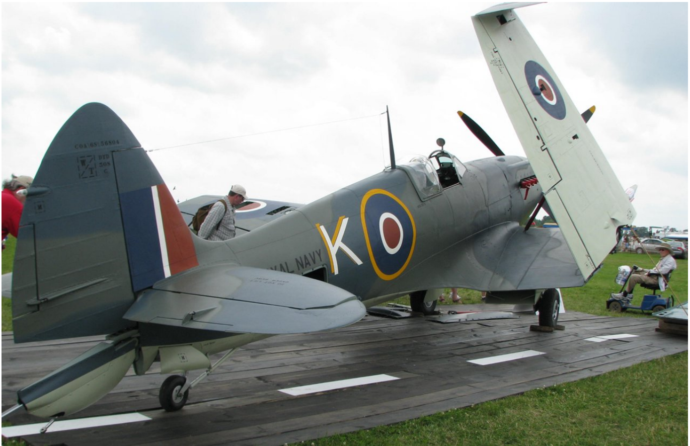
A very rare Supermarine Seafire, the carrier based version of the Spitfire, at AirVenture
