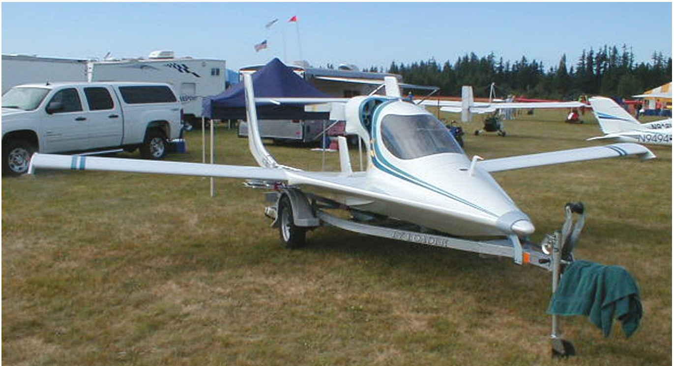
Paul Westons Sea Era single place seaplane was the hit of this year's Arlington Fly-In. It is a one off homebuilt that, besides some rakish styling, incorporates variable incidence wings to help it take off the water and also have a high cruise speed. It has flown and is his personal plane with no plans or kits to be produced.
