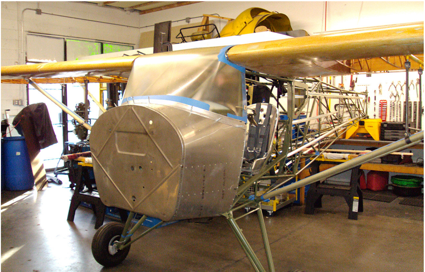
Jack Pollack's Swick T is making a visit to the Super Finishers Skunk works for final welding of the wing struts.
